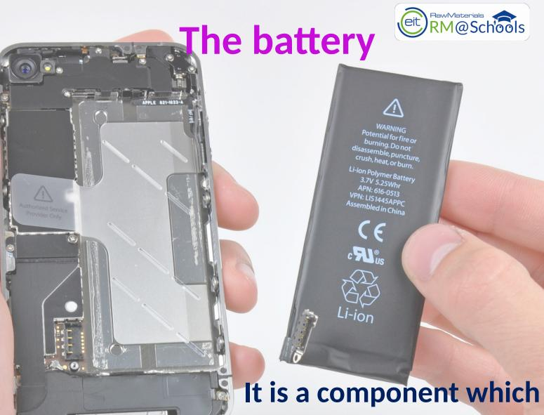
stores electricity to operate the device
