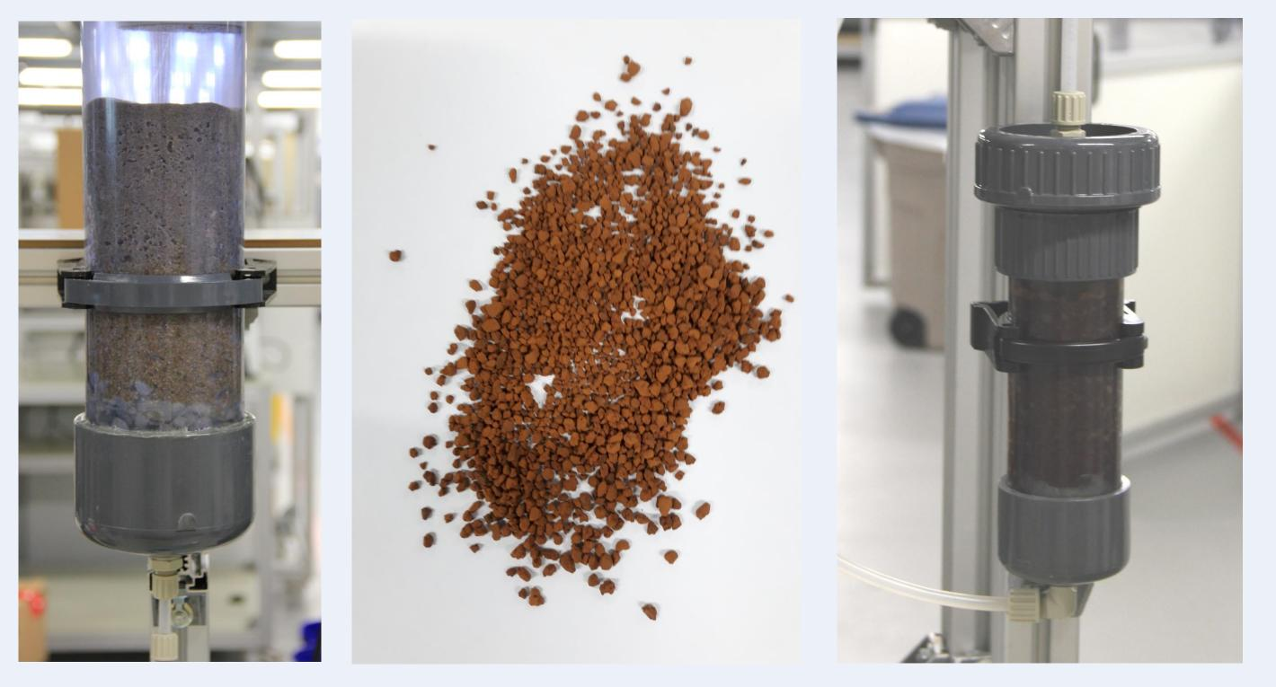
Figure 1, 2 & 3: sand filter (left), iron oxide (middle), adsorption column (right)
