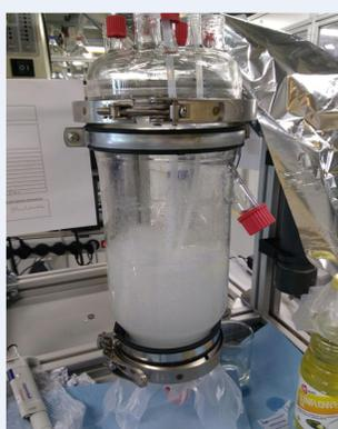
Figure 1: Airlift reactor
