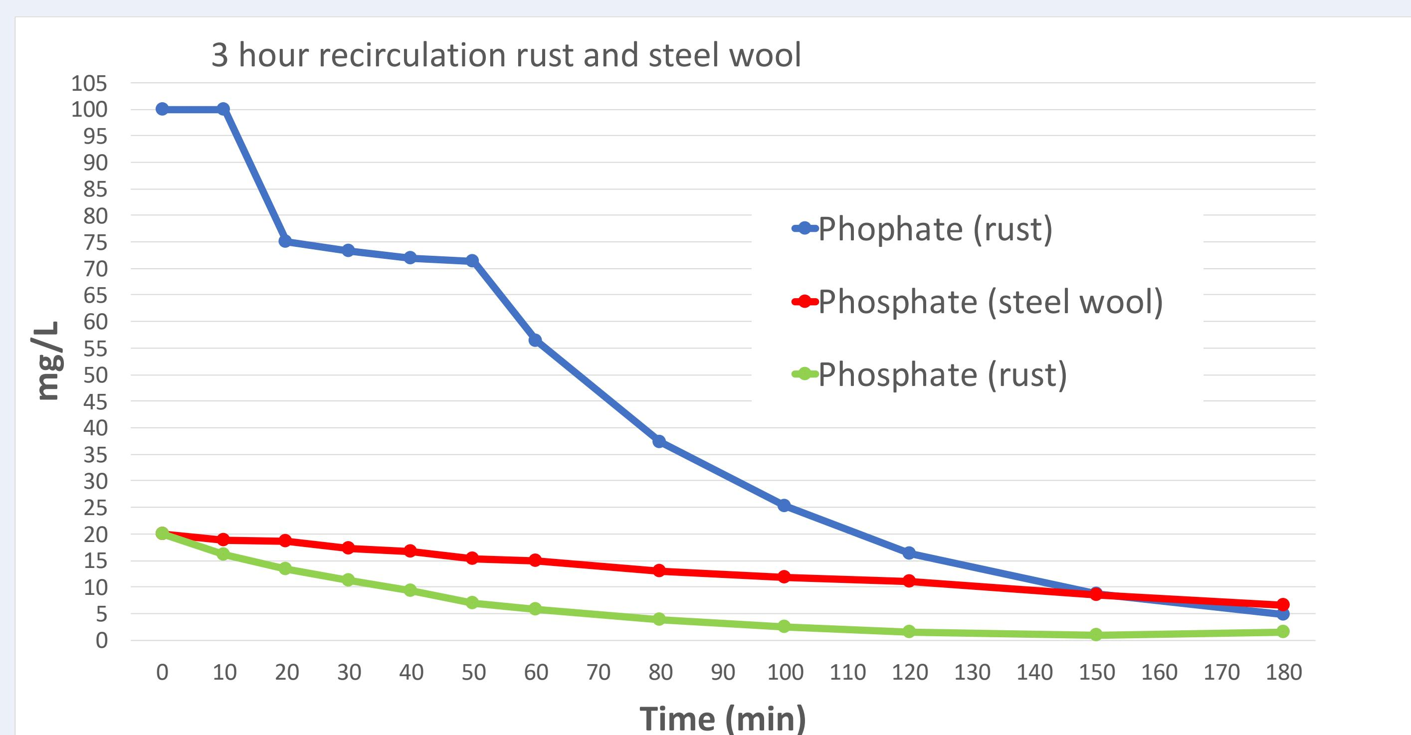
Graph 1 shows the experiment with the rust using 20 and 100 mg/L (blue and red line) and the experiment with the steel wool using 20 mg/L (orange line).
