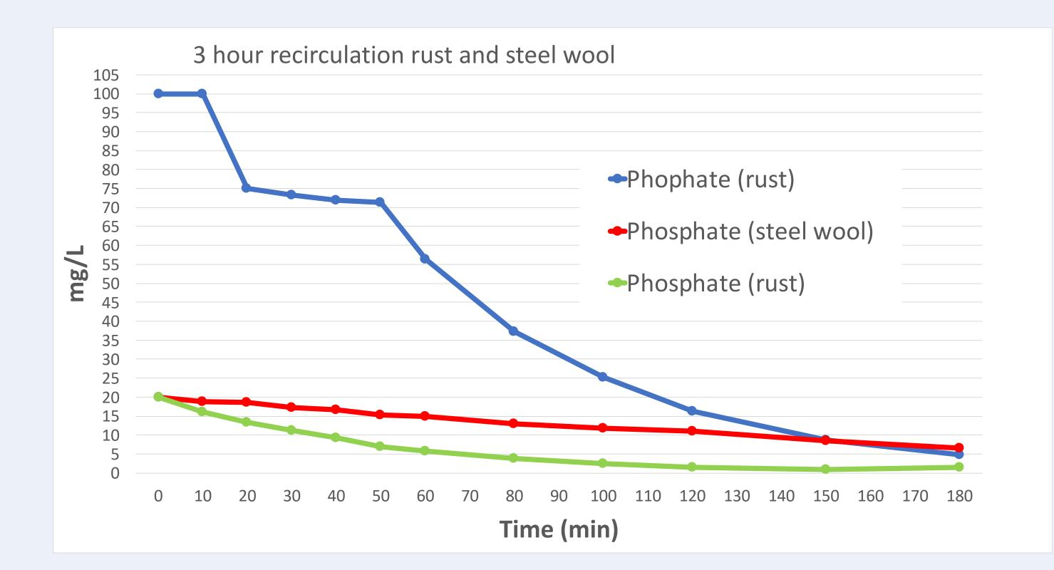
Graph 1 shows the experiment with the rust using 20 and 100 mg/L (blue and red line) and the experiment with the steel wool using 20 mg/L (orange line). As shown in the graph, the phosphate was removed in all 3 experiments. Using steel wool seems less efficient as using rust.
