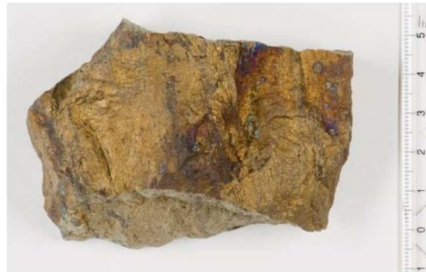
Copper ore from the sedimentary exhalative deposit at Rammelsberg , Germany. Source: Wikipedia, Hannes Grobe - Own work
