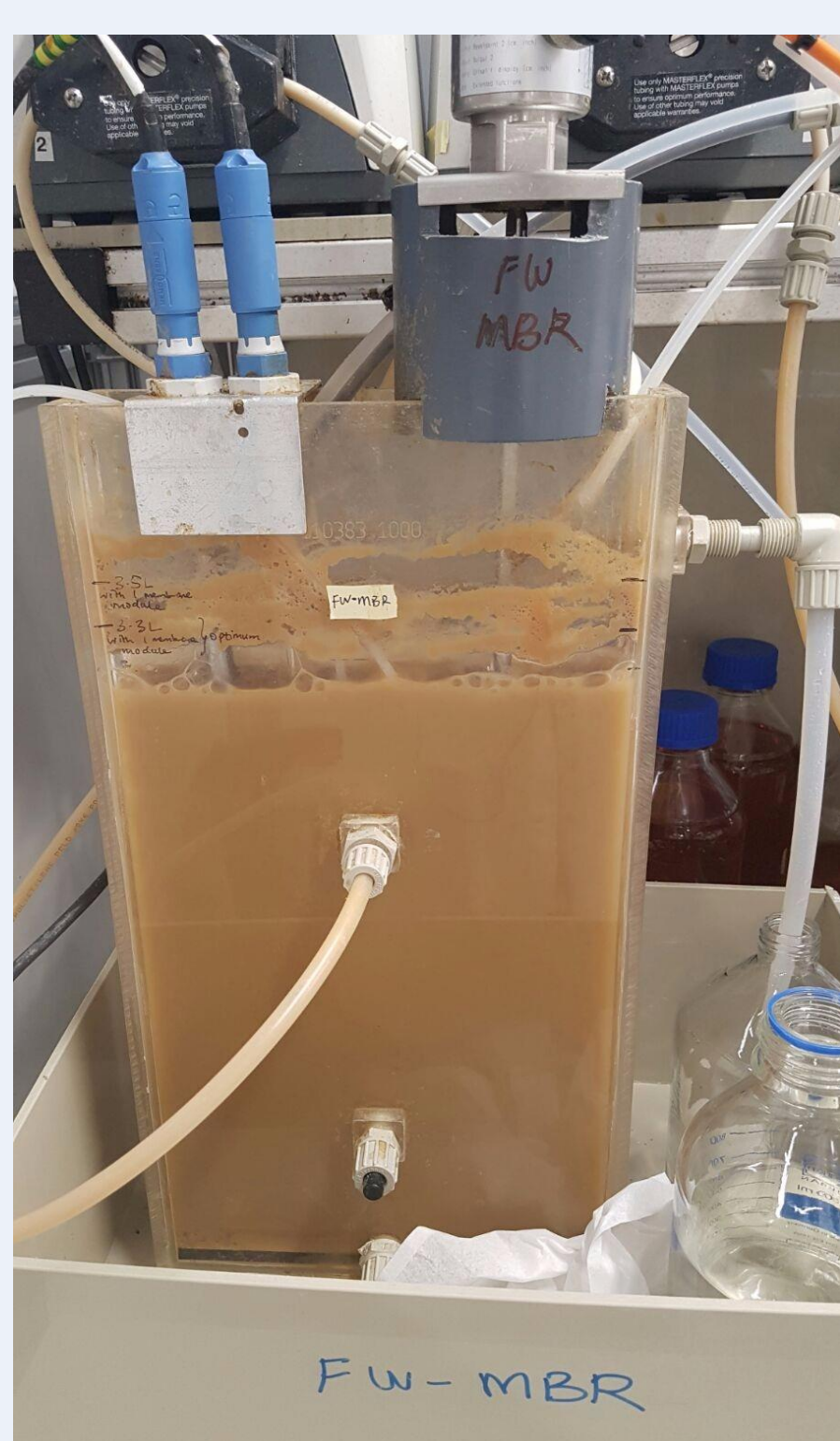
Fig. 1. Bioreactor for treating wastewater and producing EPS
