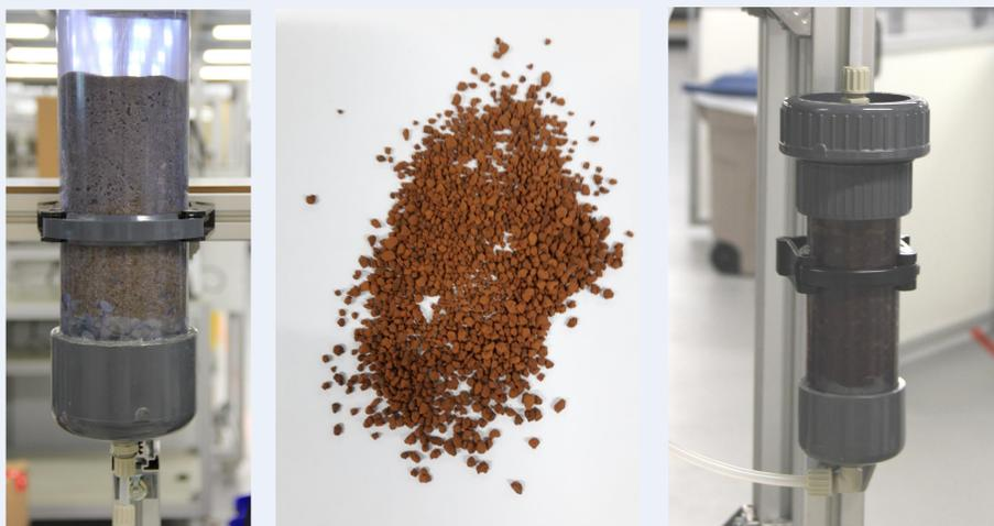
Figure 1, 2 & 3: sand filter (left), iron oxide (middle), adsorption column (right)
